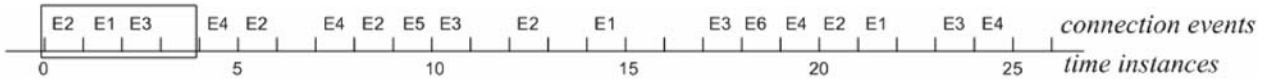
Fig. 3. Generation of a frequent episode rule by scanning a stream of Internet traffic connection events from left to right using a small scanning window.
