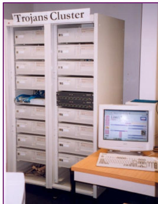
**Figure 3 The Prototype Trojans cluster built at the USC Internet and Cluster Computing Laboratory** (Visit Trojans Cluster home page: <http://andy.usc.edu/trojan/> for details)
